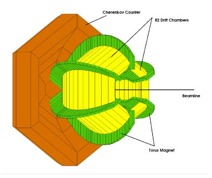
Figure 2.13: Computer rendering of the Čerenkov counter showing its position relative to the R2 drift chamber and th Torus magnet. Image source [36]
