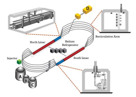
Figure 2.2: Schematic CEBAF accelerator overview, including modifications for the 12 GeV update. Image source [37]
