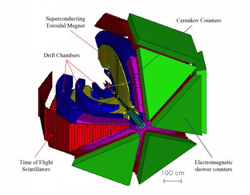
Figure 2.6: Three dimensional computer rendering of CLAS. Image source [36]
