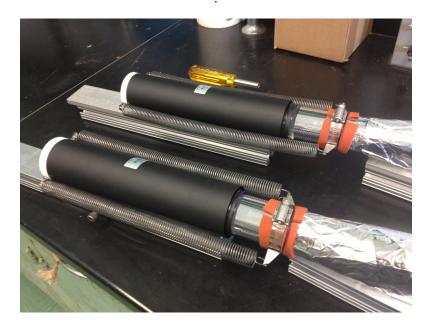
Figure B.5: The method used to attach PMT to light guides is illustrated in this photo. After the Silicon RTV was applied, the PMT/Light guide joint was held together using the device shown in this photo. Constant pressure had to be applied to the joint to ensure best results.
