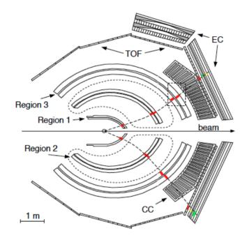
Figure 2.10: A cross sectional cut through the CLAS detector showing the position of different regions of the DC. Dashed lines outline the position of the toroidal magnet. Image source [43]
