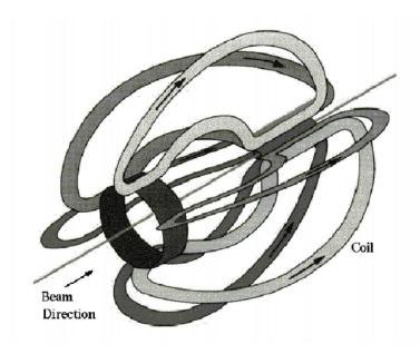
Figure 2.8: An illustration of CLAS's superconducting toroidal magnet. Image source [42]
