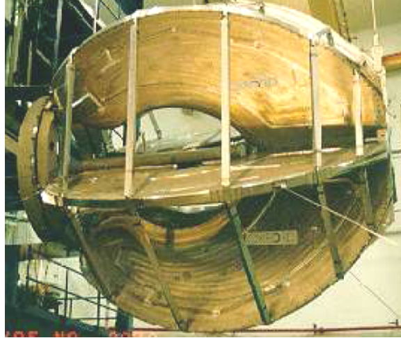
Figure 2.13: A picture of the CLAS Torus Magnet outside of CLAS during installation into Hall B. Three of the six superconducting coils of the Torus Magnet can be seen.
