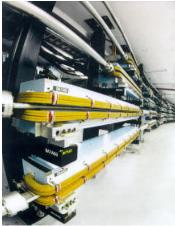
Figure 2.5: A picture of the eastern recirculation arc used at CEBAF. The yellow structures are the electromagnets used to steer the electron beam through the arc. The four different paths the electrons may take in the eastern arc are also visible.
