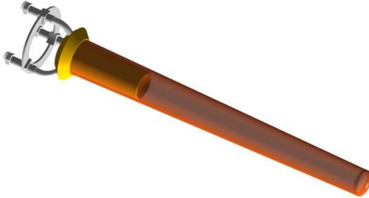
Figure 2.11: A CAD drawing of the g8b target cell. The photon beam is incident on the target cell from the left-hand side of the figure.
