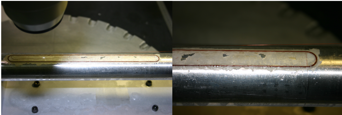
Figure A.3: A picture of the first prototype magnet showing the beginnings of one racetrack coil (a) and approximately half of one coil with two full windings (b). The white substance is purified paraffin which the wire is melted into thereby securing it in place. Visible in the right-hand side of (b) the picture is one of the semi-circles used as a template for forming the 180° turns.
