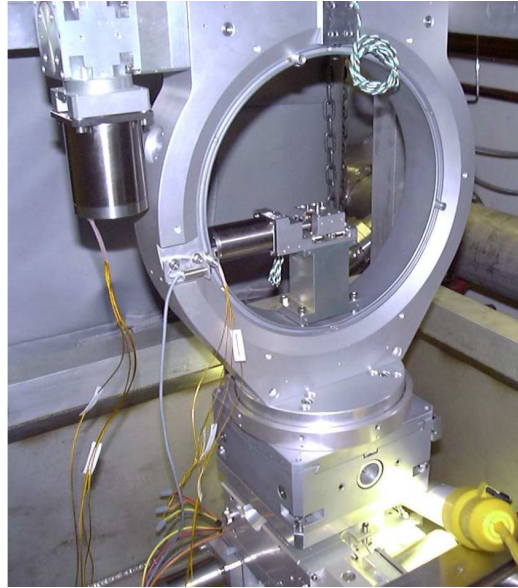
Figure 2.9: A picture of the goniometer used for the production of linearly polarized photons. In the center of the goniometer is where the target ladder is located. When used in the hall, this goniometer is positioned perpendicular to the beamline.
