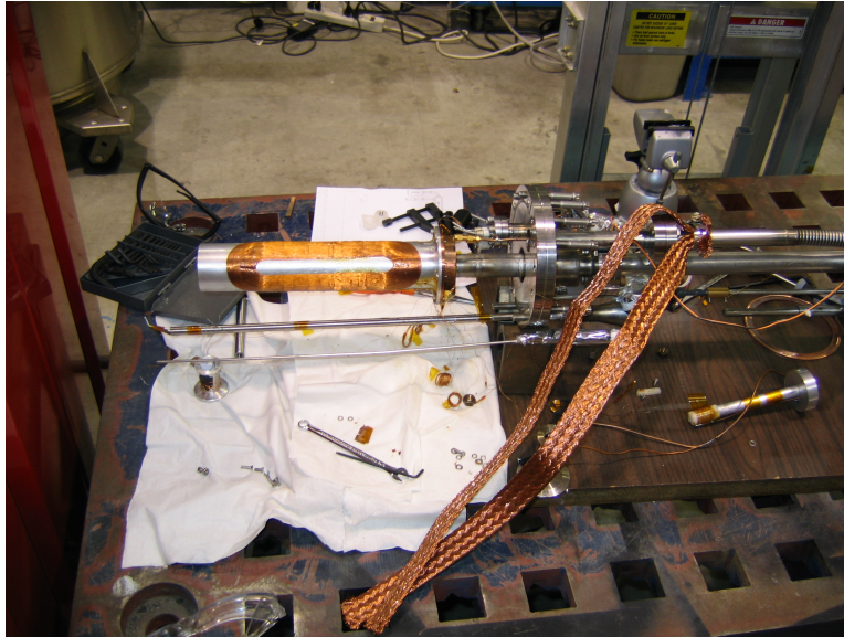
Figure A.5: A picture of the transverse holding coil produced using the semi-automated procedure. One of the two racetrack-shaped coils is visible.
