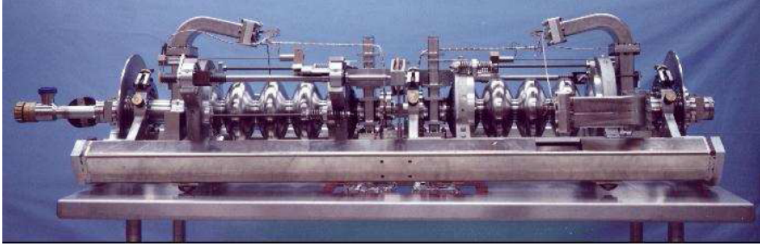
Figure 2.3: Two of the superconducting RF cavities used at CEBAF. These cavities are immersed in LHe with the elliptical cavities being perpendicular to the beamline.
