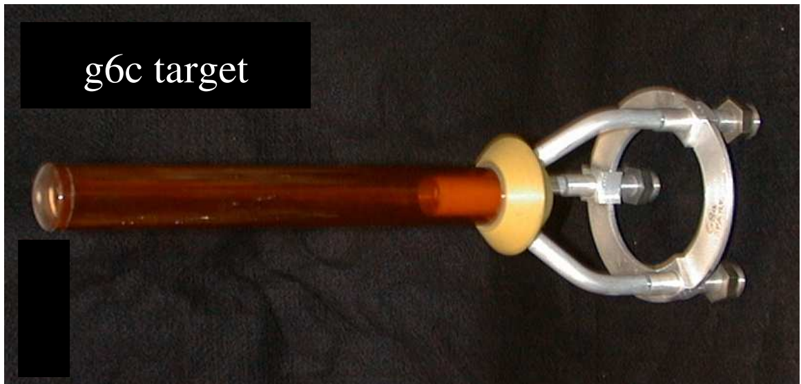
Figure 3.8. The g6c target. The cell wall is made of Kapton film. A window at each end allows the beam to pass through. The tubes at the base allow for LH_2 to be circulated into the target cell.
