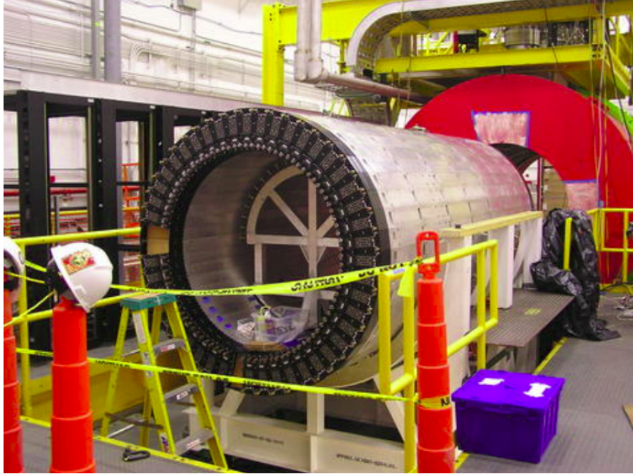
Figure 2.16: A picture of the barrel calorimeter before assembly into the superconducting solenoid. [28]
