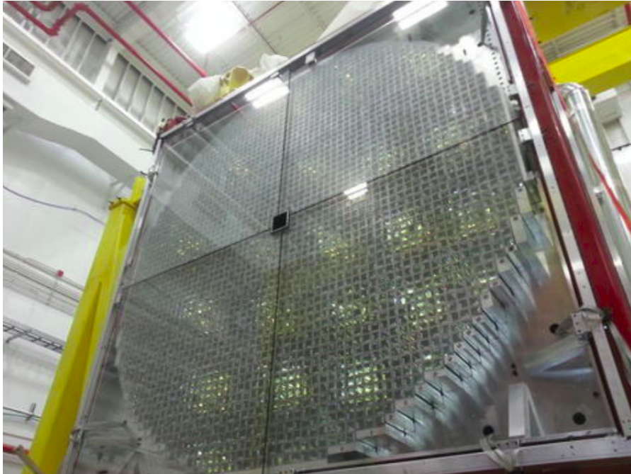
Figure 2.17: A picture of the forward calorimeter with no cover in front of it. One can clearly see the lead blocks used to reconstruct photons in the forward direction. [28]
