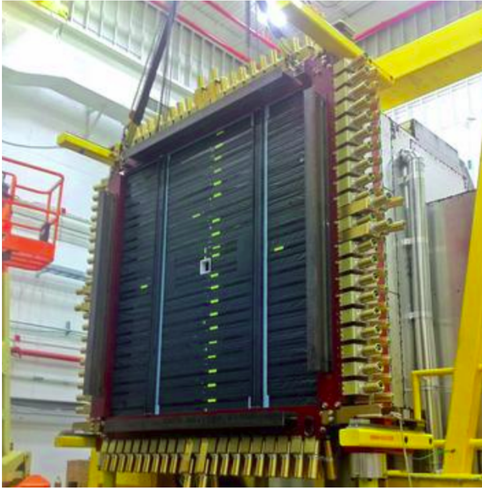
Figure 2.18: A picture of the time of flight after successful assembly inside Hall D. [28]
