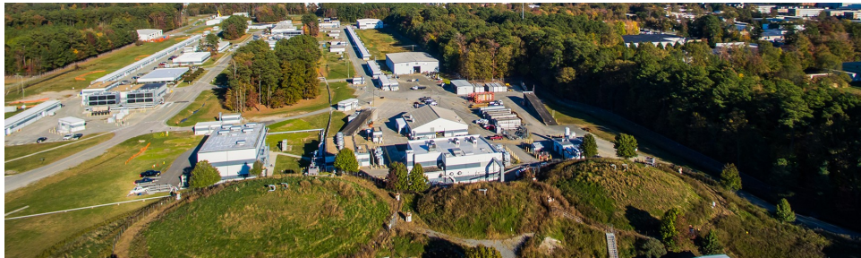
Figure 2.2: A picture taken of the Thomas Jefferson National Accelerator Facility (JLab) in Newport News, Virginia. In this picture, the electron beam from the Continuous Electron Beam Accelerator Facility (CEBAF) will travel in a clockwise motion. The two linear accelerator sections of the CEBAF are near the two parallel lab roads which run towards and away from the picture view. Three circular grass mounds can be observed in the lower part of this picture which represent the locations of Hall A, Hall B, and Hall C. Hall D is located diagonally across the CEBAF from those three halls and somewhat visible in this picture. [20]
