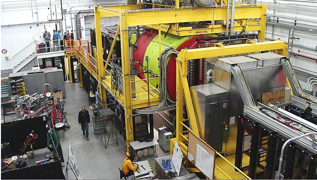
Figure 2.1: A picture taken from inside Hall D. From this angle, the photon beam would be coming towards the viewer, and eventually interact with the liquid hydrogen target located inside the apparatus. One can easily identify the shell of the superconducting barrel-shaped solenoid as well as the back side of the forward calorimeter and some photomultiplier tubes attached to the time of flight detector. [20]
